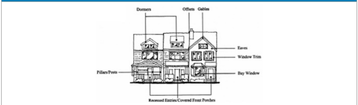
FIGURE 5.11C : ILLUSTRATION OF TOWNHOUSE BUILDING FACADE
